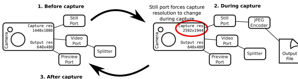
As you have probably noticed in the diagram above, the video port is a little more complex. In order to permit simultaneous video recording and image capture via the video port, a “splitter” component is permanently connected to the video port by picamera, and encoders are in turn attached to one of its four output ports (numbered 0, 1, 2, and 3). Hence, when recording video the camera’s setup looks like this:
