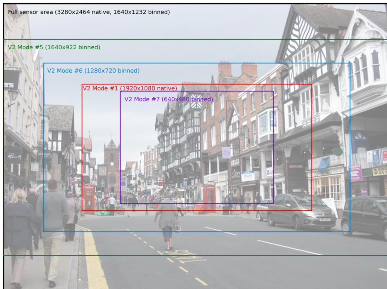
You can manually select the sensor’s mode with the `sensor_mode` parameter in the `PiCamera` constructor, using one of the values from the # column in the tables above. This parameter defaults to 0, indicating that the mode should be selected automatically based on the requested `resolution` and `framerate`. The rules governing which sensor mode is selected are as follows:
