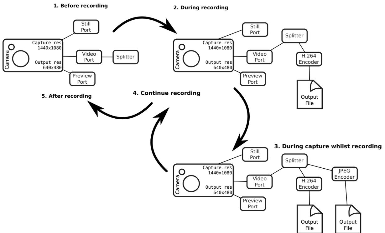
When the `resize` parameter is passed to one of the methods above, a resizer component is placed between the camera’s ports and the encoder, causing the output to be resized before it reaches the encoder. This is particularly useful for video recording, as the H.264 encoder cannot cope with full resolution input (the GPU hardware can only handle frame widths up to 1920 pixels). So, when performing full frame video recording, the camera’s setup looks like this:
