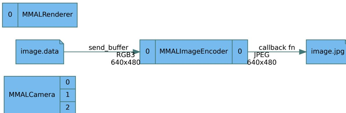
Now let's repeat the process but with the encoder attached to the still port on the camera directly. We can re-use our `image_callback` routine from earlier and just assign a different output file to `jpg_data`:
