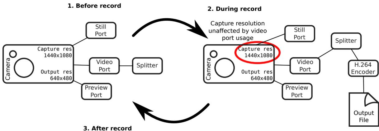
And when simultaneously capturing images via the video port whilst recording, the camera’s configuration moves through the following states:
